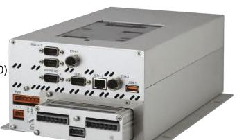
**The ELM-201 energy meter** is designed especially for energy metering on board electric traction vehicles. It can measure both the DC and AC signals of any existing traction supply system (1.5kV DC, 3kV DC, 15kV/16.7 Hz, 25kV/50Hz). Moreover, it is also suitable for multi-system locomotives using more than one electrification system.
