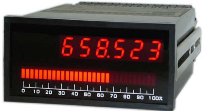
**Model OC7167** is a programmable counter with a digital display and a bargraph. The digital display has six digits. During the measurement, five digits are used with a maximum readout of 99999. All six digits are activated in programming mode. The bargraph has 30 red LEDs.
